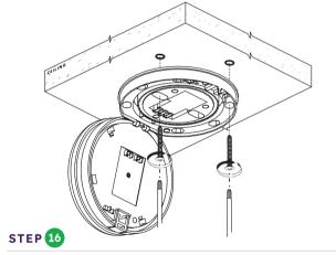
Install Alarm using provided mounting anchors and screws.
