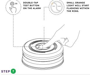
To put the smoke alarm into pairing mode, double-tap TEST button on alarm and check for a small orange light that will start flashing within the ring.
