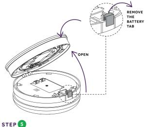
Open the Alarm and remove the battery tab.
