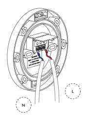
Locate compliant positions for Smoke Alarm installation(s) and attach power cables to underside of alarms, if hard wiring is required.
