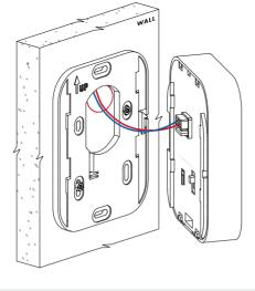
Connect the Hub cable to the power circuit wires, then connect the wired cable to the Hub.
