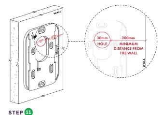
Using the mounting bracket to guide where the hole is best placed, drill a 30mm diameter hole in the wall for Hub wiring, 200mm minimum distance from the right hand side wall or other object.
